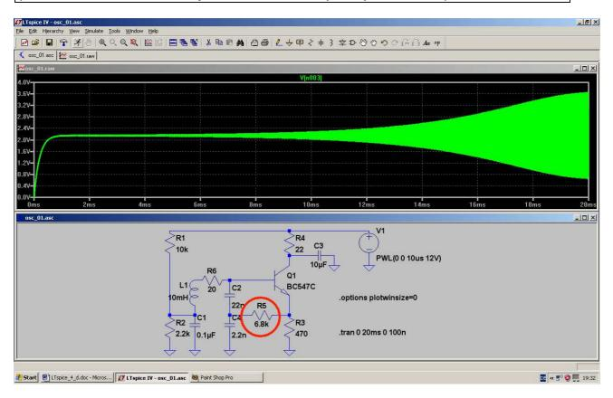
This is the result for 6.8k. The oscillation start delay is increasing....
