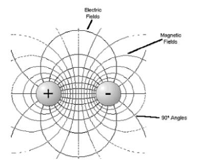
As soon as you apply a voltage to the input of a line (here the single pair is shown) you also get a magnetic field when current flows.
