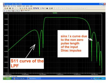
This is the result: the S11 curve of the LPF appears at the left hand side of the diagram. At the right hand side the sinx / x curve for the "spare Dirac pulse" due to its non-zero pulse length is present at high frequencies.
