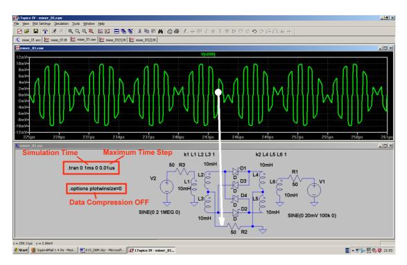
The polarity changing of the RF signal (caused by the LO signal) can clearly be seen. But: the "ON" voltage of 0.3V of every Schottky diode causes distortion at every zero crossing.
