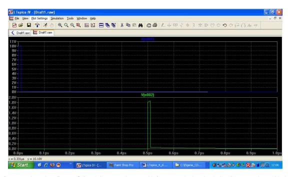
Because the value " $R = 1.7\Omega$  / 1m" does not change with frequency in the simulation (in comparison with the reality: really a pity!), all harmonics are attenuated by the same factor. So the curve form does not change as in practice (= no linear distortion). Only the amplitude at the cable's output is reduced.
