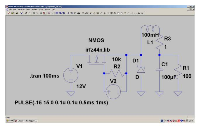
In this circuit the MOSFET serves as a switch between the power supply and the inductor and the schottky diode is connected between the node "MOSFET's source / inductor" and ground (initially reverse biased).
