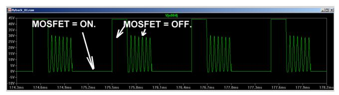
Additional information: this is the simulation with a short ON-Time (1ms) and a long OFF-Time (9ms) of the MOSFET:
