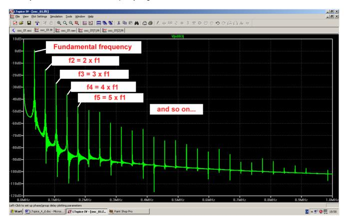
Now we can see the decreasing amplitudes of the harmonics with increasing frequency. Also the "fundamental oscillating frequency" can now be determined more accurately as 35.7kHz.
