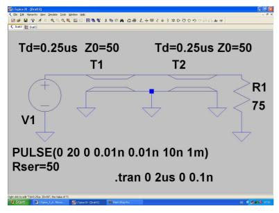
We terminate the end of the cable by a  $75\Omega$  resistor and simulate a run time of 2ms (...please check all of the schematic before starting the simulation...):
