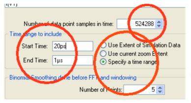
Here come the necessary entries for the FFT. Do not forget to ignore the time range from 0....20 ps with the input pulse and use 524288 samples.
