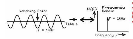
Only a pure continuous sine wave where neither the start point nor the stop point can be observed consists of only one spectral line!
