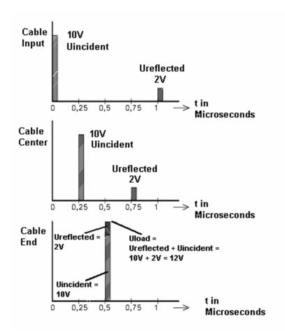
At the cable input we see at first the incident wave (produced by the pulse generator) with an Amplitude of +10V.
