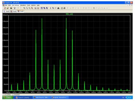
The linear frequency spectrum simulated with 131,072 samples is shown here.
