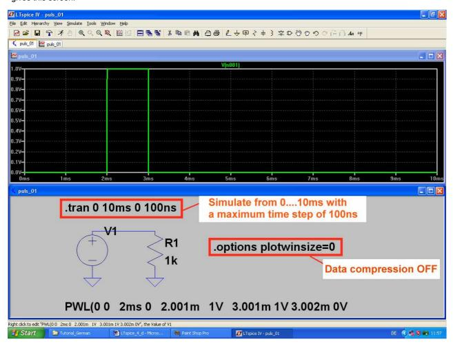
Now we want to perform a Fast Fourier Transformation and so some explanation is necessary: Choosing a simulation time of 10ms is crucial for the FFT simulation result because you get from it the lowest frequency of the spectrum AND the frequency resolution (...including the line width of a signal...) by the following relationship:
