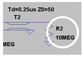
Change the termination to  $10M\Omega$  -- this will do for an ideal open circuit.
