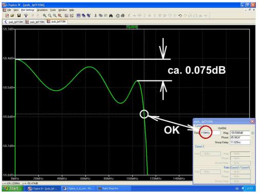
The ripple corner frequency value with 110MHz is correctly simulated, but there is an error of 0.075B at the Chebychev ripple calculation.
