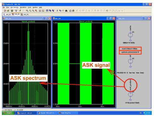
The spectrum of the ASK signal is shown in Fig 22, it shows what was to be expected. The symmetrical square wave information signal contains the 1KHz fundamental and all odd number harmonics. The result is LSBs and USBs with all these spectral lines of the information signal that spread to the left and right of the carrier.
