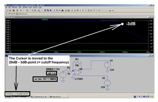
Using the cursor you will find the corner (= cutoff) frequency at 75.6kHz. Here the gain has decreased by -3dB.
