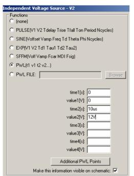
To start the (simulated) oscillation the circuit needs a little "push". This is done by programming a special property of the supply voltage:
