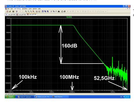
This is the simulation result for a linear frequency axis:
