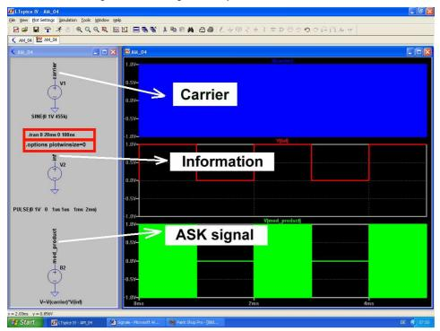
A carrier signal of 455kHz was selected for this example. This figure shows the simulation circuit with the output signals of the three voltage sources used with a peak value of 1V or 0.707V RMS.
