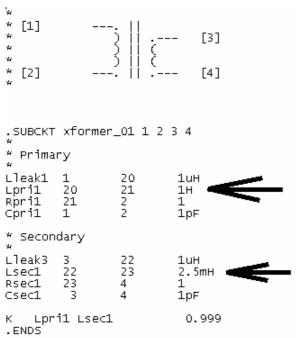
For an ideal transformer you can reduce the values for the flux leakage inductances, the copper resistors and the winding capacitances.
