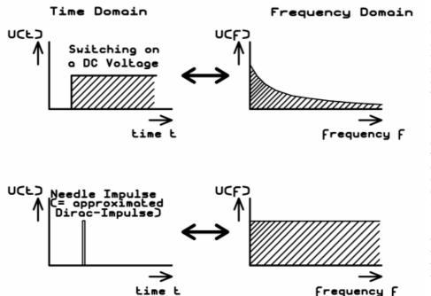
Switching On or OFF of a DC voltage gives a spectrum with decreasing spectral power density at increasing frequencies.
