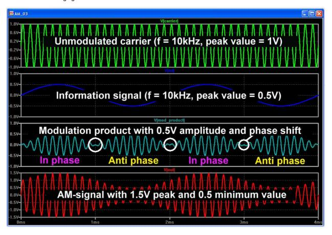
The top trace shows the constant 10kHz carrier with a peak value of 1V. Below that is the information that is a 500Hz sine wave with a peak value of 0.5V. If these two signals are multiplied the result is a signal at the carrier frequency where:
