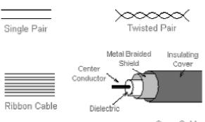
The "Single Pair" is simple: two wires held in parallel.
