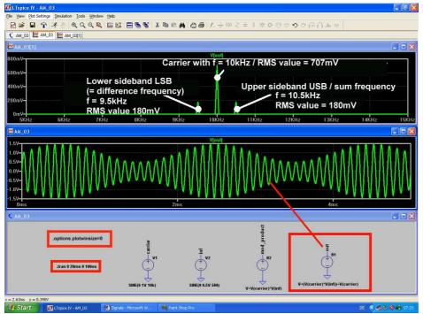
For the complete AM signal the carrier signal is added to the modulation product. This can be simulated using the by source as shown in this figure.
