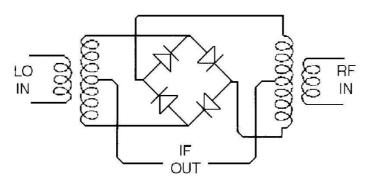
A ring of four schottky diodes is connected to two transformers. Each transformer uses 3 identical windings. The two secondary windings are connected in series.
