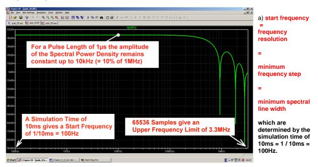
b) The upper frequency limit in the diagram (= stop frequency) is determined by the number of samples used for the FFT **AND** by the maximum time step (which gives the minimum sample frequency in the time domain).
