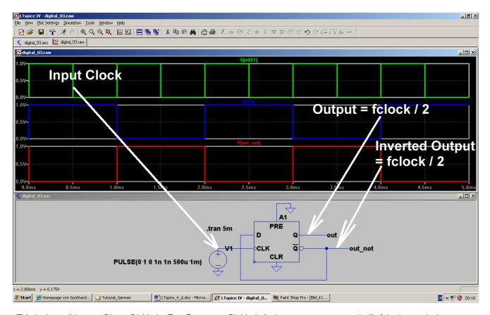
This is the well known "Binary Divide by Two Frequency Divider". At the output you get one half of the input clock frequency. The inverted Q-output is connected to the D-input pin.
