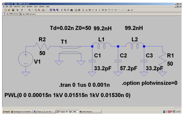
Voltage source V1 is connected to the input of a  $50\Omega$  cable with a signal travelling time of **20 picoseconds** (= part "tline" in LTspice). The output of this cable feeds the input of the LPF with the Dirac impulse (amplitude = 1 kiloVolt, pulse length = 15 picoseconds, rise and fall time = 0.15 picoseconds, start at t = 0). The following value pairs are used to generate this impulse:
