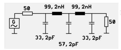
...and these were the part values calculated by a LCfilter design program.
