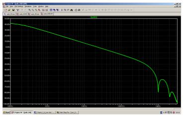
At higher frequencies the influence of the "single Dirac impulse" can be seen. This means that we see the Sinx / x – envelope with zeros belonging to the NON-ZERO pulse length. So do not use the results in this region.
