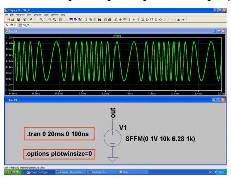
Take a close look at this figure. The frequency of the signal increases during the negative half wave and decreases during the positive half wave of the information signal. Unfortunately the modulating information signal cannot be shown on a separate diagram in this mode. Data compression is switch off as usual. It is simulated over 20ms (100ns resolution) but for clarity only a short section is shown. The rest can be seen from the SFFM source programming. The line:
