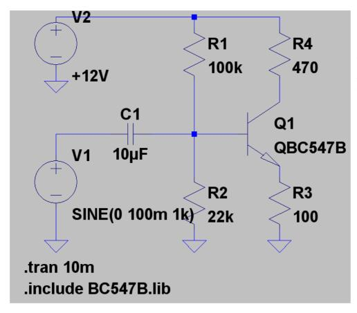
We need a power supply, a sine voltage source, one capacitor, four resistors and an npn-transistor.
