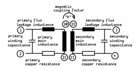
Node 1 and 2 are the primary winding connections, node 3 and 4 the connections for the secondary winding of the model for the simulation. For the "inner nodes" you should choose much higher numbers to avoid collisions when "blowing up the circuit diagram" with more windings ore parts.
