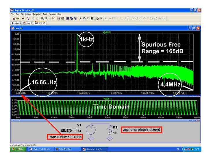
It is true! From 17Hz up to 4.4MHz every undesired signal is attenuated by more but 160dB and only the 1kHz sine wave line can be seen. Nearly ideal and perfect...
