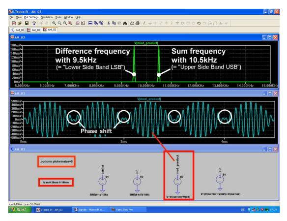
To simulate this we use the Behavioural Voltage (bv), this has the necessary tools to simulate the multiplication of the two signals. This is confirmed in the above figure:
