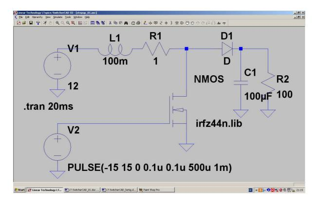
The schematic shows a +12V power supply , followed by an inductance with L = 100mH and the obligatory series resistor of  $1\Omega$ .
