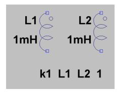
Example for a two winding transformer and voltage transfer ratio = 1.1
