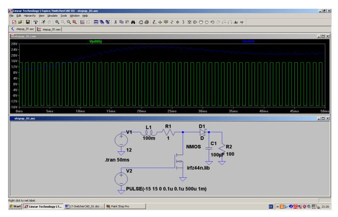
Clearly, it can now be seen that the output voltage is a mixture of a mean DC Value of +23V and a small "sawtooth-ripple" (= charging and discharging of the output capacitor).
