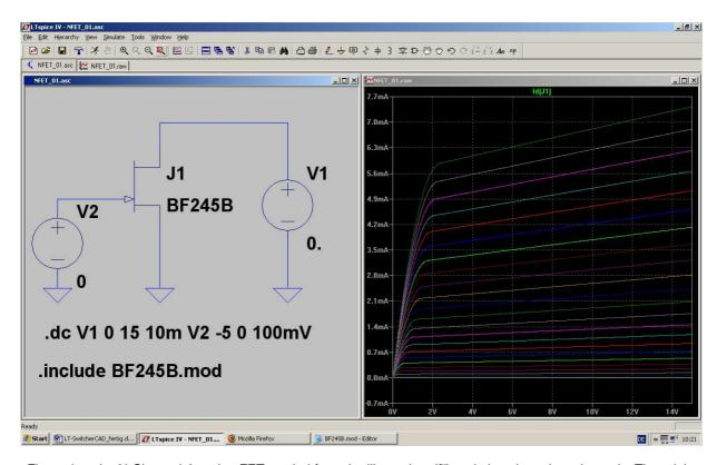
First select the N-Channel Junction FET symbol from the library (= "njf") and place it on the schematic. Then right click on the model description "NJF" beside the symbol. Change it to **BF245B** and finally add a SPICE directive to the schematic:
