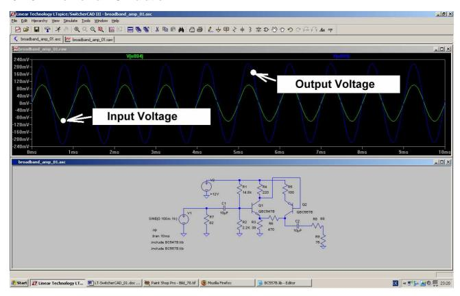
As required the output voltage's peak value is twice that of the input voltage and that gives a gain of 6 dB..... Two common emitter stages produce a phase shift of  $2 \times 180 = 360$  degrees. So the output voltage is again in phase with the input voltage.
