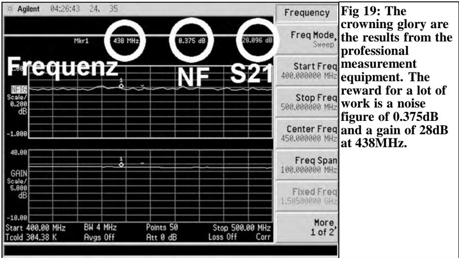
**Fig 19: The crowning glory are the results from the professional measurement equipment. The reward for a lot of work is a noise figure of 0.375dB and a gain of 28dB at 438MHz.**
