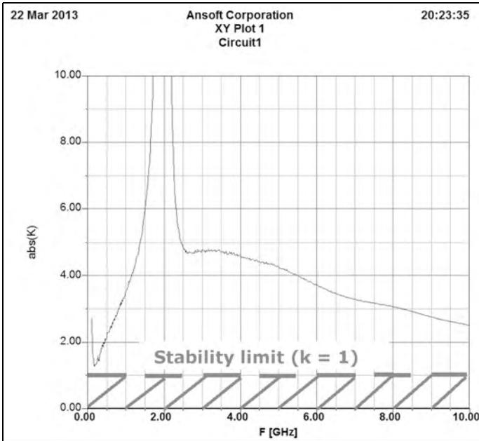
**Fig 10:** The modified circuit has a positive effect on the stability.
