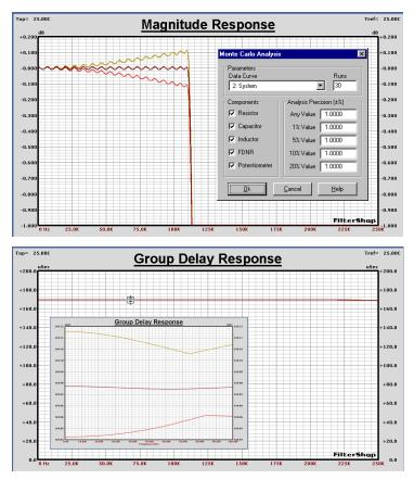
The magnitude response shows up to a  $\pm 0.1$ dB deviation as the frequency approaches the high passband edge at 110kHz. The group delay shows little relative effect, while the enlarged insert does show that small variations do indeed occur.
