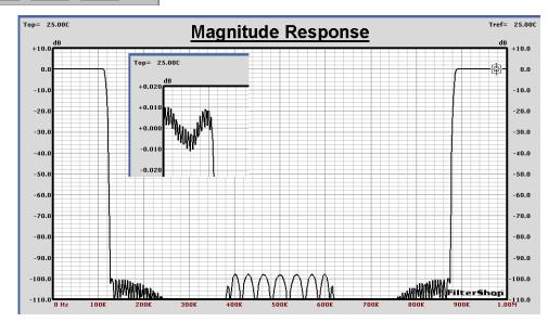
The passband/stopband regions cover the same frequencies as before, but the stopband now shows the combined response of two different FIR filters.
