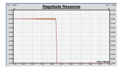
An alternative approach which does not require ultra high precision components is a *trim pot* for calibration. The sensitivity analysis showed that all of the R/C components had roughly the same unity sensitivity on controlling the response. For small changes in any component value, an almost linear relationship exists for changes at the output.
