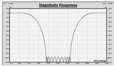
Both of the two FIR filters are providing stopband attenuation, but indifferent frequency regions. The best choice of FIR order for each of the two stages was determined by the Multirate dialog.
