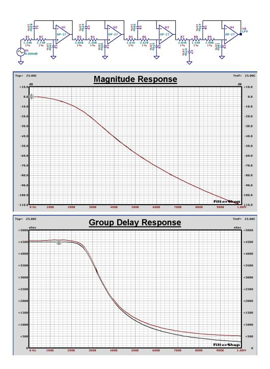
We are not that concerned with the actual level of the delay, but that the delay remain flat in the 110kHz passband. Since the circuit wants to produce more delay, we must provide it with a new objective target curve that it can match.
