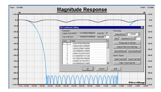
Decimation causes the higher frequencies to fold back into the output spectrum. This folding is based on the output sample rate, in this case 40kHz. In order to keep the desired bandwidth of 0Hz - 5kHz clean, the filter must remove all higher frequency regions which would fold back across the 5kHz band.
