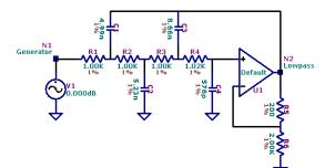
To change the gain back to unity, R1 will be increased slightly and a resistor added to ground. We will also want to use 10% standard values for the capacitors. The opamp will be changed to a 5534 type.
