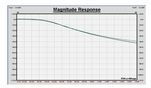
The optimization frequency range is initially the entire 160kHz bandwidth, with all components at 1% precision. Compensation for the opamp finite bandwidth will require changes in the capacitor values. In order to determine what the best range is for the capacitors, all of the components are optimized except for R5 and R6.
