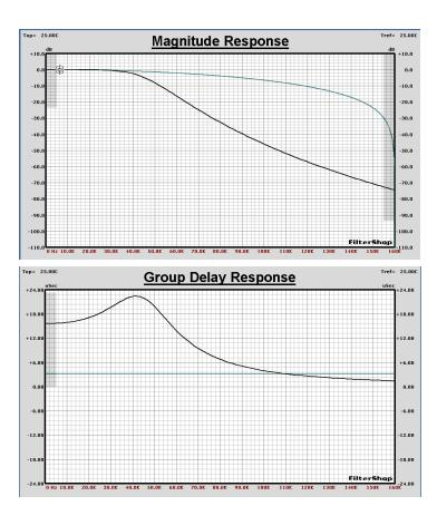
A Butterworth-6dB was chosen since this provides a compromise between the Bessel and standard Butterworth-3dB. A 7th order LP with Fo=47kHz was chosen. The response is shown here in Black.
