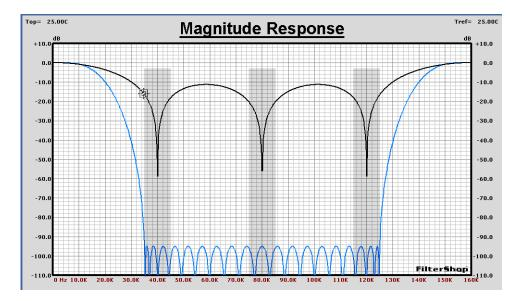
Each repetitive null of the comb filter lies exactly on top of all the regions which must be removed. However, the intersection of the comb filter response at the edges of the gray regions is only 15dB down. Clearly this does not meet the design objective.
